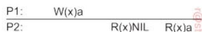
Figure 7.4: Behavior of two processes operating on the same data item. The horizontal axis is time.
